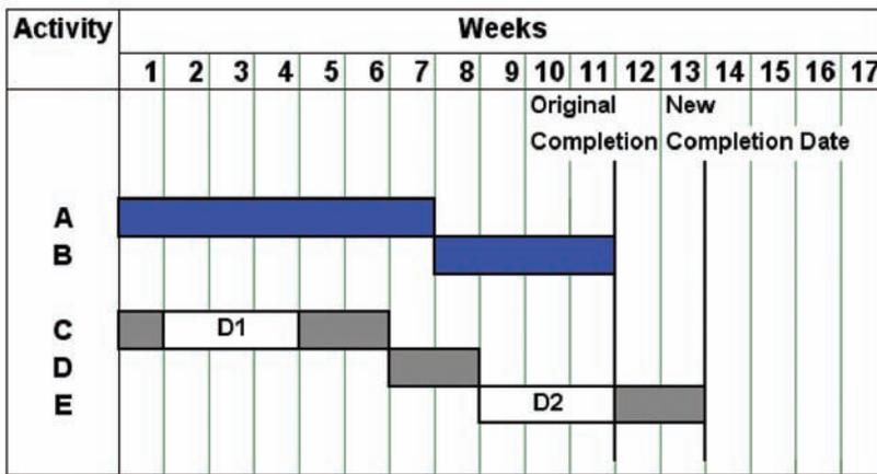
**Figure F - Scenario 2d for D2 delay absorbed by D1 delay.**
